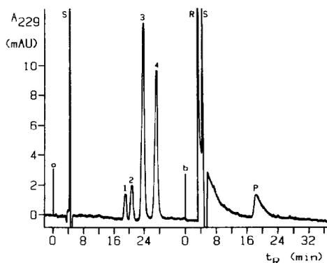
Fig. 4. Extraction of PG/PDC reaction mixtures with ethyl acetate. (a) Organic phase, (b) aqueous phase, both reconstituted after removal of ethyl acetate under nitrogen. Conditions as in Fig. 2, except detector with 2- $\mu\text{l}$  flow-cell. Peaks: 1, 2, 3 and 4: 15-oxo-PGF<sub>2a</sub>, -PGF<sub>1a</sub>, -PGE<sub>2</sub> and -PGE<sub>1</sub>, respectively; R = reagent; S = solvent; P = pyridine.
