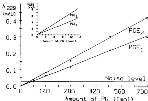
Fig. 5. External calibration of oxidized standard PGE<sub>2</sub> and PGE<sub>1</sub>. Noise level as indicated at  $3 \cdot 10^{-5}$  a.u.f.s. peak-to-peak. Chromatographic conditions as in Fig. 2. Injected volume, 1 µl.
